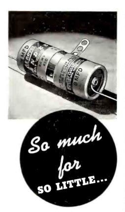
\* Originally introduced by others as a purely price proposition, the miniature-can electrolytic has become the practical and dependable DANDEE. Adequate dry section; true hermetic sealing; proper safety venting; spunover jacket ends to eliminate shorts; polarity-indicating end washers; conservative ratings—these AEROVOX features have justified these generalutility electrolytics for normal-duty service.
