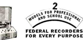
The Symphonic Model Federal Recorder, designed for profes-sional use, incorporates many new and exclusive features. Records on all size disks up to 16-inch. Overhead, fully adjust-able cutting head. Speed-governor turntable. Records over microphone and radio simultaneously. Operates at 78 or 33½ RPM. Complete with dynamic microphone, floor stand and cord.
