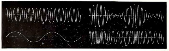
(a) Radio carrier wave of constant amplitude.(b) Audio (or program) wave for modulating (a).
