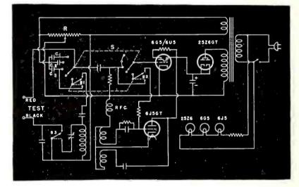
Schematic of the BQC Solar capacitor checker which uses Wein bridge and RF oscillator in compact unit.
