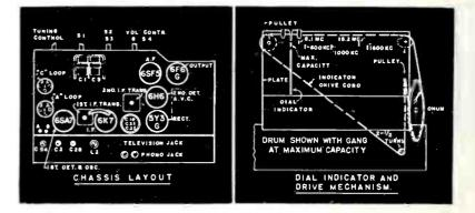
Top view of chassis and front of dial cord plate for RCA K61
