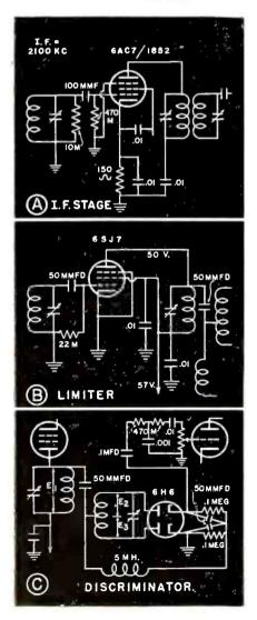
further smooth out the resonant peak in the IF transformer, a loading resistor of 10,000 to 15,000 ohms is used across the secondary. This loading resistor has the effect of making the total impedance reflected back into the primary consist of more resistance and less reactance. The variations of capacitive and inductive reactance over the range of 200 kc. is therefore made less effective in determining the transformer gain.
